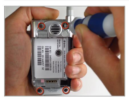
Unscrew the four 6mm long screws with a Tri-Wing Y1 screwdriver.
