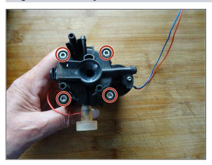
• Unscrew the four Torx T20 screws holding the ceramic valve together.
