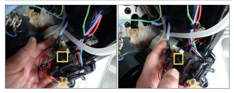
• Pull off the clamps on the other two pressure hoses. Make a note of which hose goes where and detach the two hoses.
