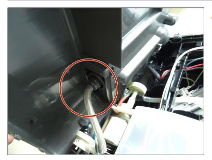
• Pull off the silicone hose that leads to the water connection of the tank from the inside.
