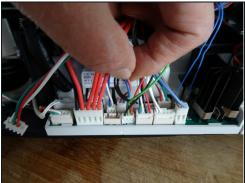
• Locate the two strands of wire going from the ceramic valve to the motherboard. Unplug the connectors and unthread the cables.
