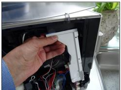
• If you haven't already done so: Remove the two plastic covers over the cables and the electronics box.
