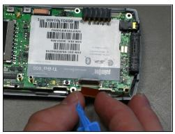
⚠ Disconnect the ribbon cable before removing the motherboard.
