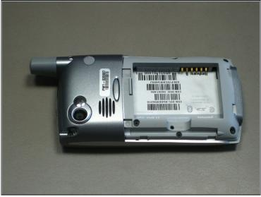
• Lift the edge of the battery, separating contact points, and pull out as pictured.
