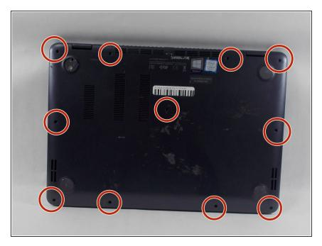
Use a Phillips #00 screwdriver to remove the ten 6.4 mm screws from the bottom cover.
