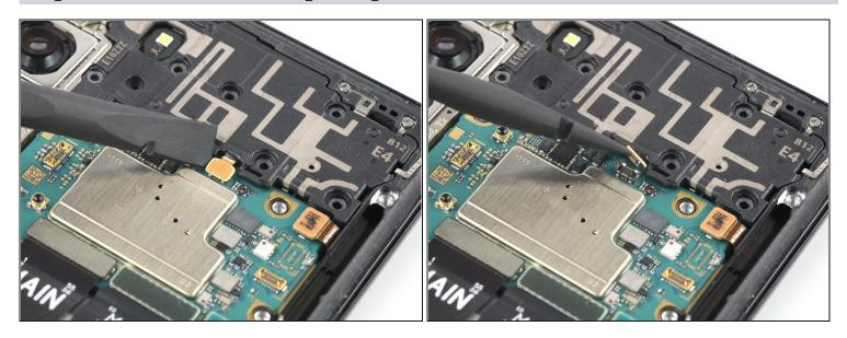
• Use a spudger to disconnect the earpiece speaker cable by prying the connector straight up from its socket.
