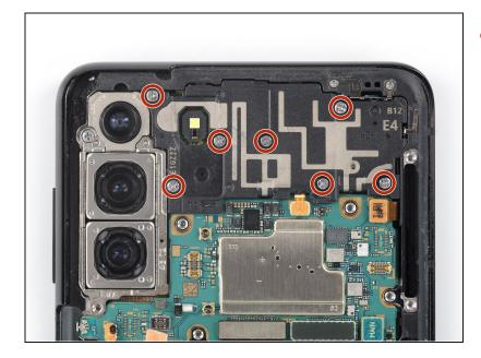
Use a Phillips screwdriver to remove the seven 3.9 mm-long screws securing the earpiece speaker assembly.
