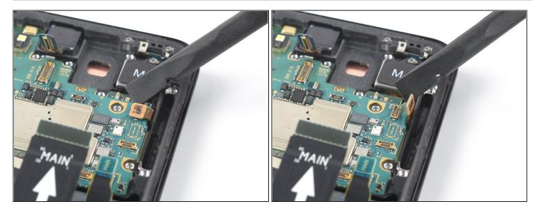
⚠ During the following step do not fold the cable sharply and only bend it to avoid cable damage.
