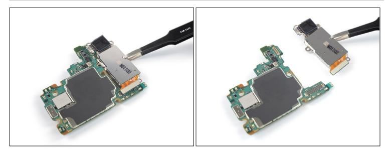
• Use a pair of tweezers or your fingers to carefully separate the camera assembly from the motherboard.
