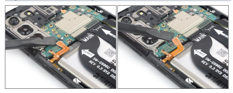
• Use a spudger to disconnect the battery cable by prying the connector straight up from its socket.
