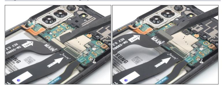
• Use a spudger to disconnect the display flex cable by prying its upper connector straight up from its socket.
