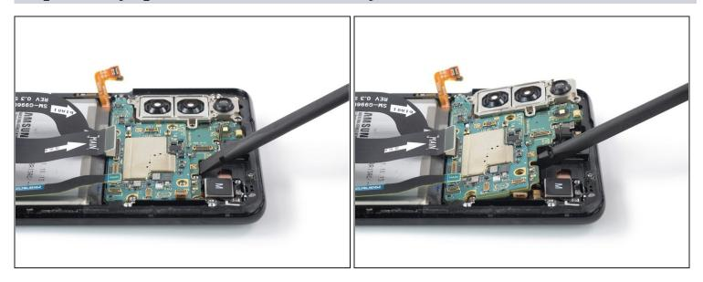
A Make sure no cables are tangled with the motherboard assembly during the removal procedure to avoid cable damage.
