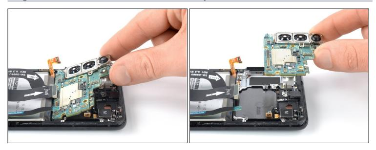
• Carefully remove the motherboard assembly including the rear cameras.
