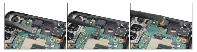
• Use a spudger to disconnect the front facing camera cable by prying the connector straight up from its socket.
