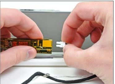
• Disconnect the white inverter cable from the right end of the inverter board.
