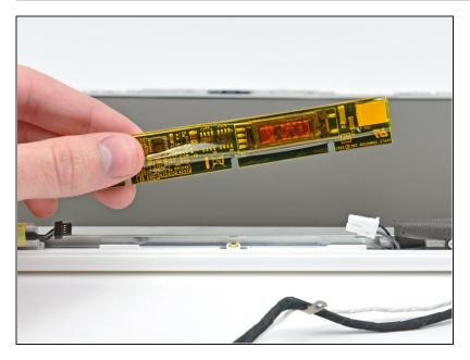
Remove the inverter board from the display.
