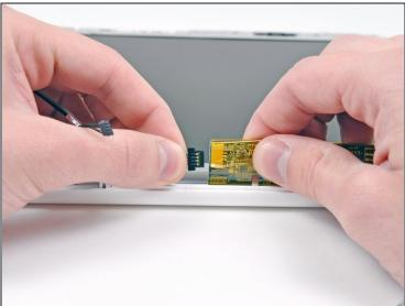
• Slightly lift the newly-revealed inverter board out of its housing and disconnect the black inverter cable from the left end of the board.
