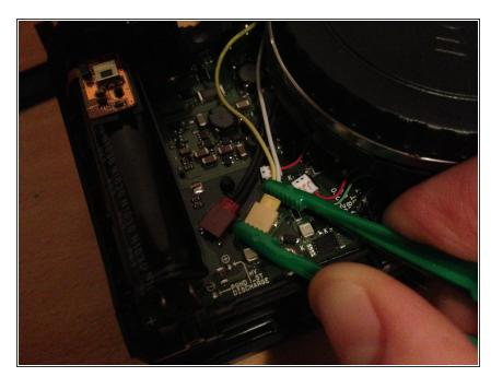
Reattach the red and yellow connectors on the front of the camera. Be sure to route the cables so they cannot interfere with the front cover when replaced.
