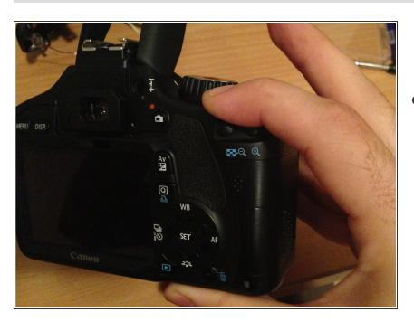
Gently place the back onto the camera as you removed it. Squeeze down gently but firmly until top cover and back are in place and screw holes are aligned.
