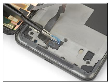
Use tweezers to remove any tape from the display connector cover.
