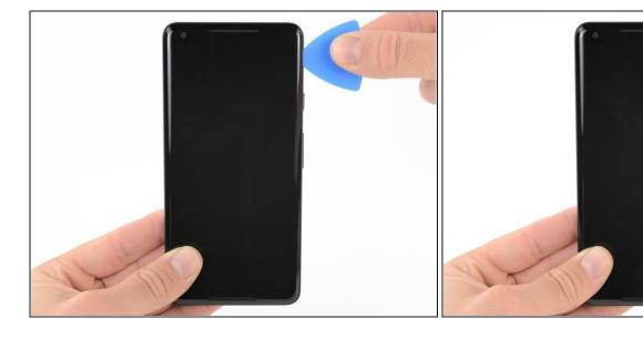
Slide the opening pick down the right side of the phone to separate the display adhesive.
