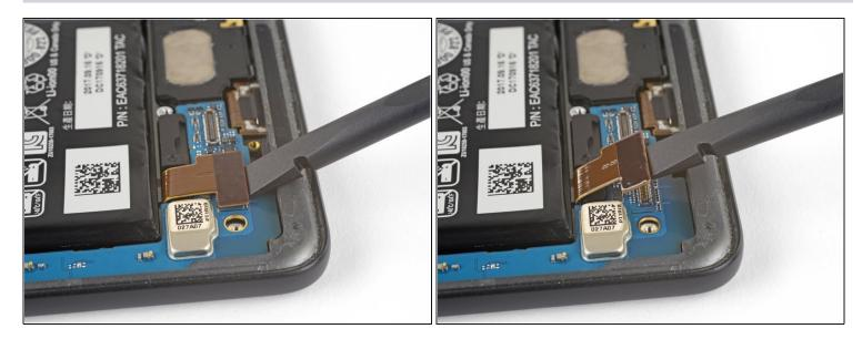
Use the flat end of a spudger to disconnect the charging assembly connector.
