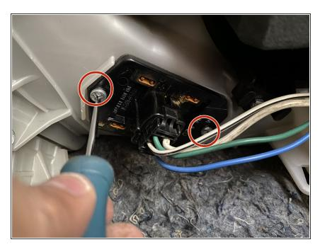
Remove the two 1 mm Phillips #0 screws that secure the blower motor wiring harness.
