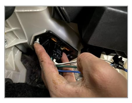
Tighten the two 1 mm screws to the wiring harness.
