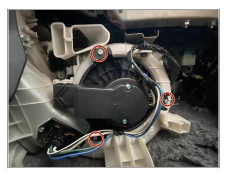
Remove the three 2 mm screws that secure the blower motor.
