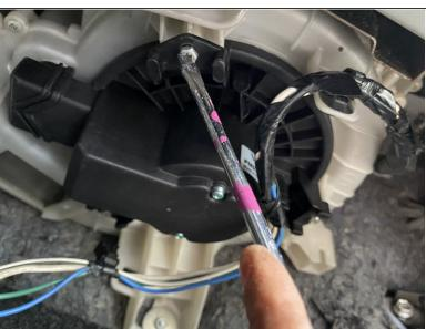
Put the new blower motor in place, and secure it with the three 2 mm Phillips #0 screws.
