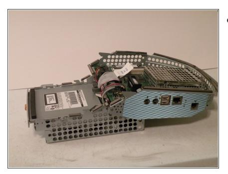
The logic board assembly. This is the heart of the computer, it contains the motherboard, CPU, RAM, V-RAM, PRAM battery, the hard drive, and the optical drive.
