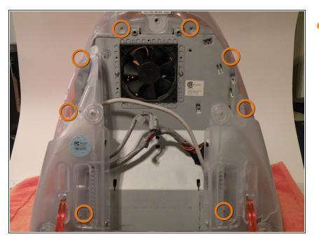
To remove the bottom cover, remove these phillips screws, and pull the bottom cover off the iMac. (Start with the very back and use a flat head screwdriver to pop the main clip. The rest will come off relatively easily.)
