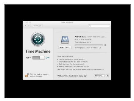
Quick update: the Time Capsule will easily accept a <u>4TB 3.5" hard drive</u> in place of its *lowly* 2TB original drive. The Seagate was used to take this screenshot, but the HGST drive should work fine as well.
