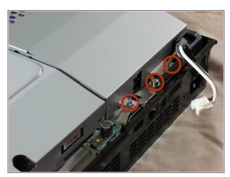
Remove the screws on the back of the power supply with a Phillips #2 screwdriver.
