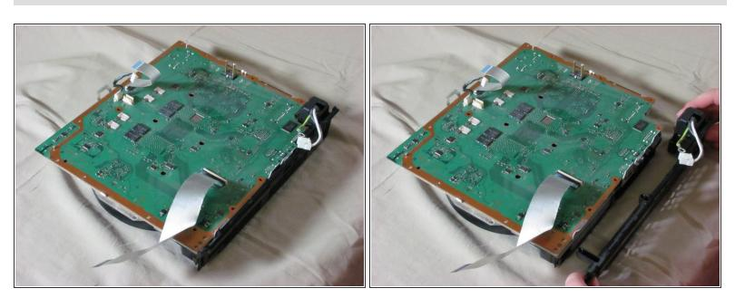
Slide the back panel out of the enclosure.
