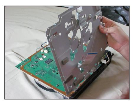
Remove the large, top plate by tilting it back until it comes off.
