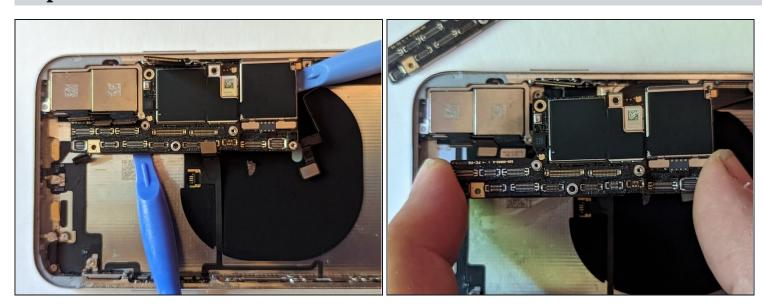
• The logic board assembly is mounted on two posts going through the lower board and are secured to the upper board. In order to remove it, you must lift it evenly straight up to clear the stand-offs.
