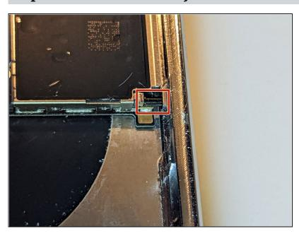
• When the SIM card is ejected, a pin slides out from the frame and pushes on the eject lever in the SIM card carrier. The pin needs to be pushed back into the frame so it will not block the removal of the logic board.
