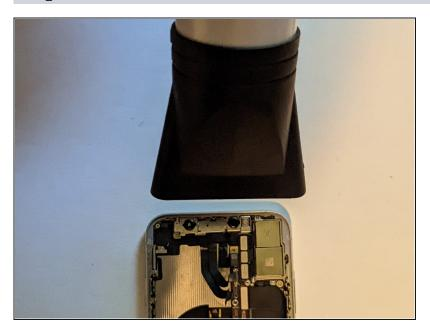
Apply heat to loosen the adhesive on the front camera assembly.
