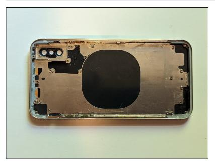
The case has been stripped completely of all parts. You can now replace them into a new case.
