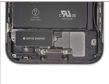
• Remove the 2.1 mm Y000 screw securing the speaker connector cover.
