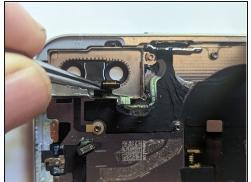
• Peel the flex cable from the frame.
