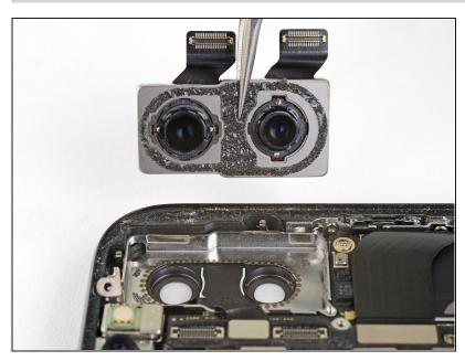
• Remove the rear-facing camera module.
