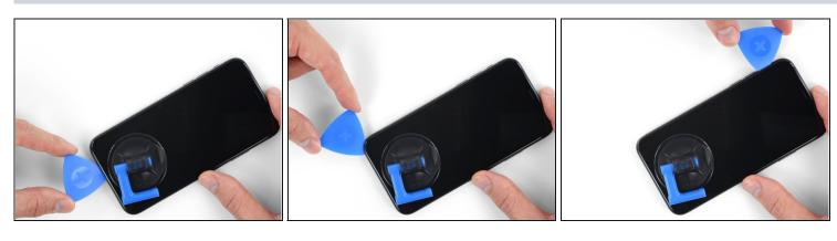
Slide the opening pick around the lower left corner and up the left edge of the iPhone, slicing through the adhesive holding the display in place.
