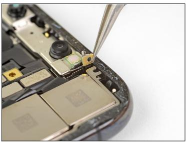
• Use tweezers to gently fold the small metal grounding bracket out of the way. Do not pull up on it as it is connected to a fragile flex cable.
