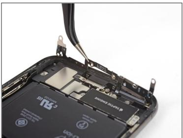
• Lift the bracket from the edge nearest the battery. Don't try to remove it fully, as it's still connected via a small flex cable.
