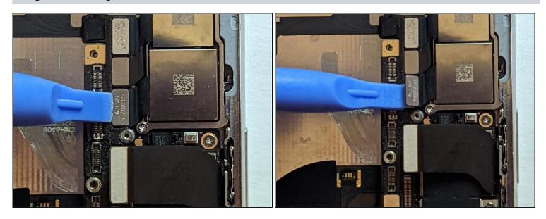
• Disconnect the Telephoto Camera cable connector.
