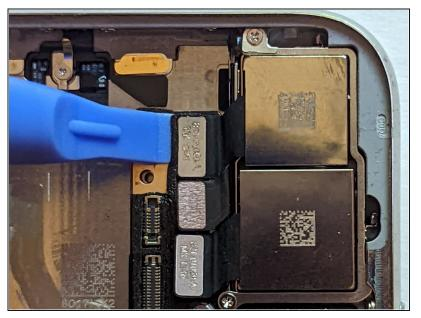
• Disconnect the Wide-Angle Camera cable connector.
