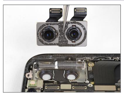
• Remove the rear-facing camera module.
