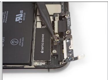
• While holding the bracket out of the way, use the point of a spudger to pry up and disconnect the flex cable underneath.
