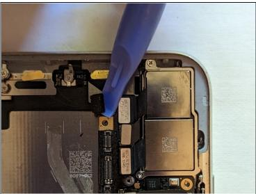
• Disconnect the WiFi Antenna cable connector.
