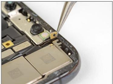
• Use tweezers to gently fold the small metal grounding bracket out of the way. Do not pull up on it as it is connected to a fragile flex cable.
