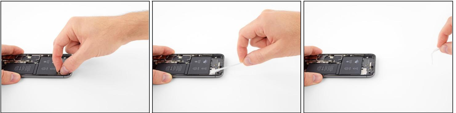
**i** In the following steps, you'll pull each tab to slowly stretch out the adhesive underneath the battery. This special stretch-release adhesive loses its tack when stretched and then comes out in your hand, allowing you to lift out the battery with ease.
