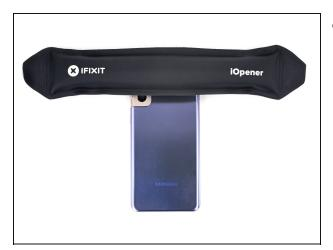
Heat an iOpener and apply it to the top edge of the back cover for two minutes.
