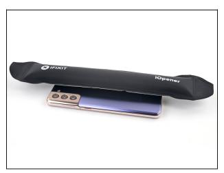
Heat an iOpener and apply it to the right edge of the back cover for two minutes.
