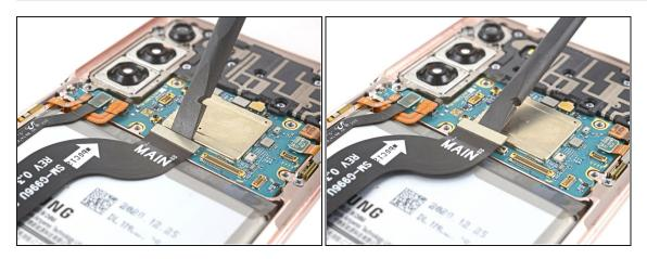
• Use a spudger to pry up and disconnect the display cable's press connector.
