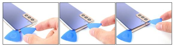
⚠ When you slice near the camera assembly, insert only the tip of the opening pick (~4-5 mm) to avoid damaging or smearing the camera.
