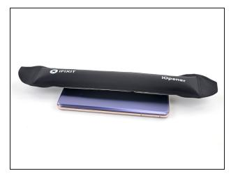
Heat an iOpener and apply it to the left edge of the back cover for two minutes.
