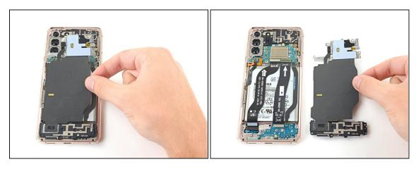
• Use a pair of tweezers or your fingers to carefully remove the NFC antenna and charging coil assembly.
