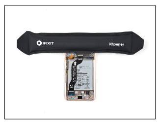
Apply a heated iOpener to the front camera for 90 seconds.
