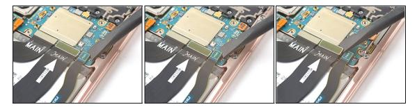
• Use a spudger to pry up and disconnect the primary and secondary interconnect cables' press connectors on the motherboard.
