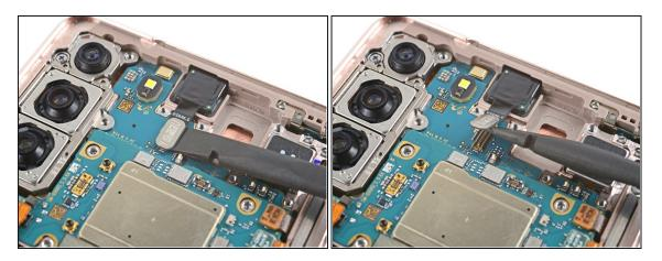
Use a spudger to pry up and disconnect the front camera's press connector.
