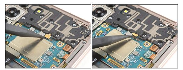
• Use the tip of a spudger to pry up and disconnect the earpiece speaker's press connector.
