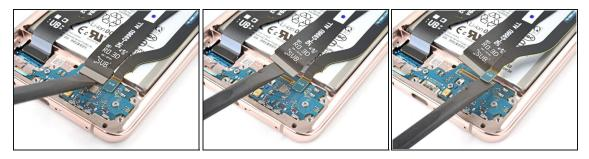
• Use a spudger to pry up and disconnect the primary and secondary interconnect cables' press connectors on the daughterboard.
