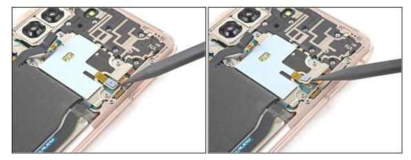
• Use a spudger to disconnect the NFC antenna by prying the connector straight up from its socket.
