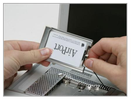
• Hold the Airport card in one hand and use your other hand to remove the antenna cable.
