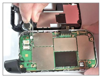
Using tweezers, pull with gentle pressure in the direction of the wire to unplug from the motherboard connector.
