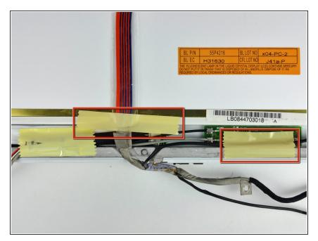
Remove the two pieces of tape over the display data/microphone cables near the lower edge of the display.
