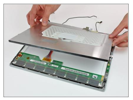
• Lift the thin steel LCD cover off the LCD.
