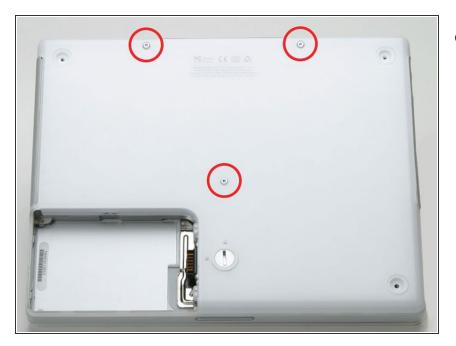
Remove the one 10 mm and two 20 mm hex screws using a 2mm hex.
