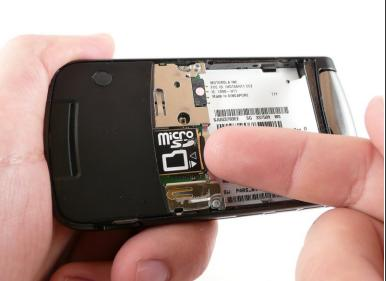
Press the exposed portion of the SD card towards the bottom of the phone until you hear a click.
