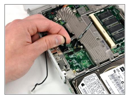
Use the black plastic handle to disconnect the display data cable from the logic board by pulling straight up.
