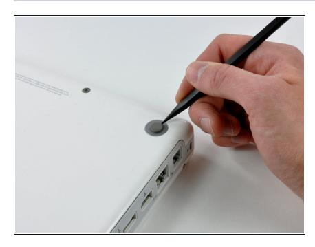
Use a spudger or small flathead screwdriver to remove the three rubber feet from the lower case.
