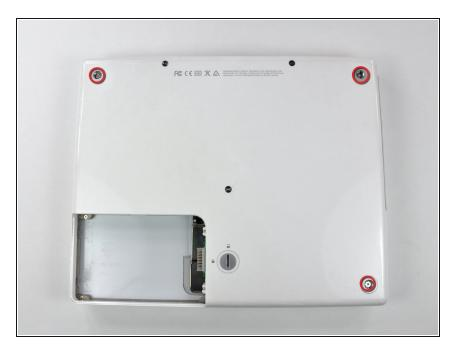
Remove the three newly-revealed Phillips screws.
