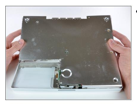
• Lift the bottom shield off.
