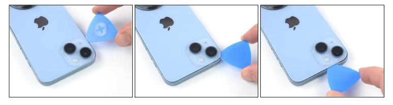
• Insert your pick underneath the top-left edge of the phone. Slide it around the top-left corner and halfway across the top edge.
