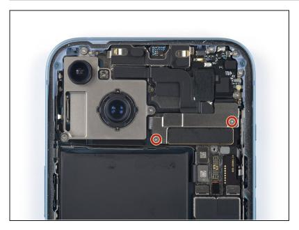
Use a Y000 screwdriver to remove the two 1.3 mm-long screws securing the front camera assembly cable bracket.
