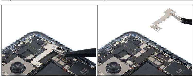
• Use a pair of <u>tweezers</u> or your fingers to remove the front camera assembly cable bracket.
