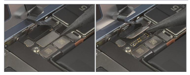
• Use the pointed end of a spudger to disconnect the charging coil cable by prying the connector straight up from its socket.
