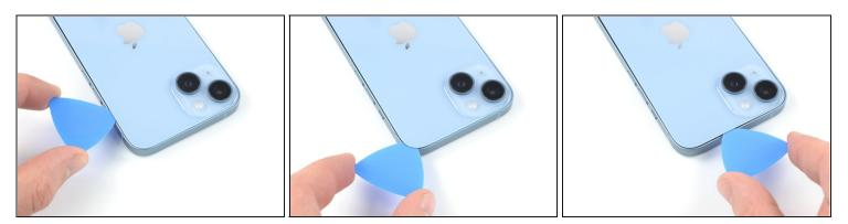
• Insert your pick underneath the top right edge of the phone. Slide it around the topright corner and halfway across the top edge.
