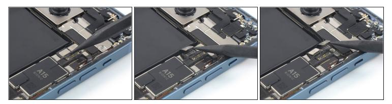
• Use a spudger to disconnect the two rear facing camera cables by prying the connectors straight up from their sockets.
