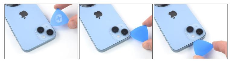
• Insert your pick underneath the top-left edge of the phone. Slide it around the top-left corner and halfway across the top edge.
