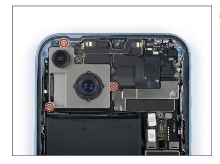
• Use a Phillips screwdriver to remove the three 2.1 mm-long screws securing the rear camera assembly.
