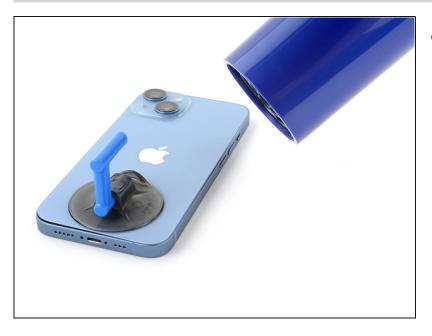
• Use a hair dryer to heat the right edge of the iPhone (the edge with the power button) for 90 seconds or until the rear glass is slightly too hot to touch.
