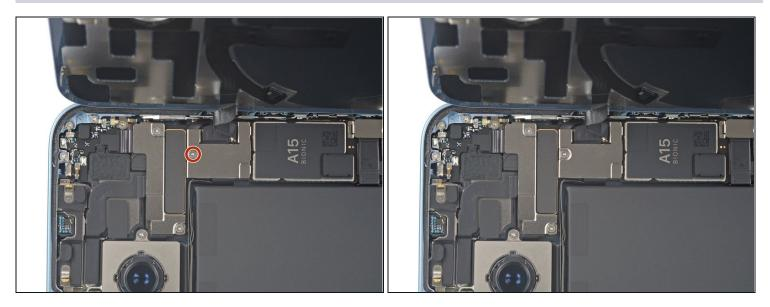
• Use a Y000 screwdriver to remove the single 1.0 mm-long screw securing the charging coil connector cover.
