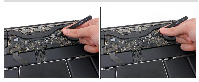
Use tweezers to remove the small plastic cover located near the bottom right of the battery connector board.
