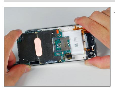
Slide the logic board towards the dock connector and out of the iPhone.
