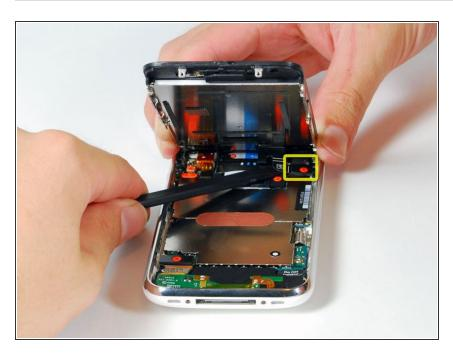
Continue to hold the display assembly with one hand, and use your other hand and a spudger to disconnect the black ribbon cable labeled "1."
