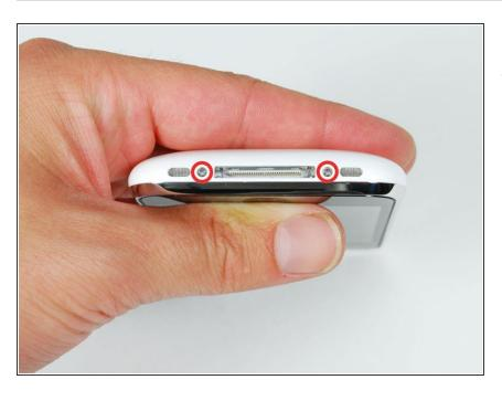
Remove the two Phillips #00 screws from the dock-connector end of the iPhone.
