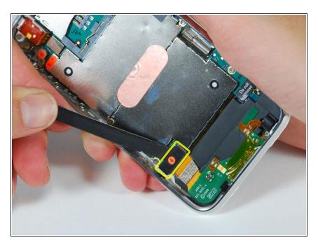
Use a spudger to disconnect the ribbon cable labeled "4."
