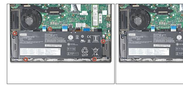
• Use a Phillips #0 screwdriver to remove the five 5.2 mm-long screws securing the battery.
