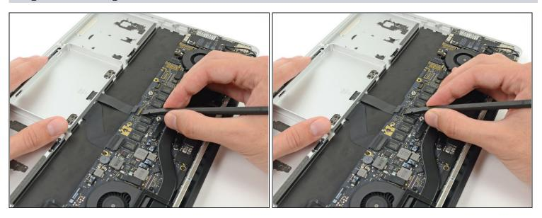
• Use the flat end of a spudger to flip up the retaining flap on the trackpad ribbon cable ZIF socket.
