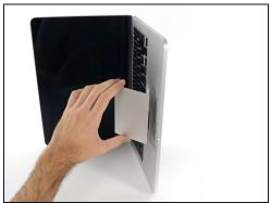
Gently pull the trackpad from the upper case, being careful not to snag the ribbon cable.
