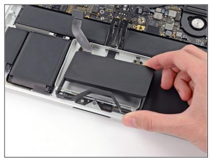
• Remove the SSD assembly from the upper case.
