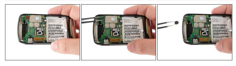
• Use a pair of <u>tweezers</u> or your fingers to remove the small rubber cap from the motherboard.
