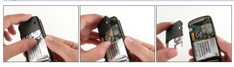
• Tilt the loosened half of the rear housing away from the phone. The housing should easily separate after tilting it about 45 degrees away from the phone.
