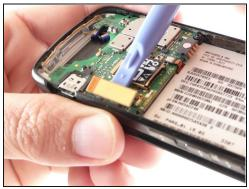
• Use a plastic opening tool to gently pry the main motherboard cable connector away from the RAZR2.
