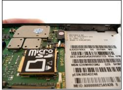
• Use a spudger to flip open the white clamp holding the keypad ribbon in place.
