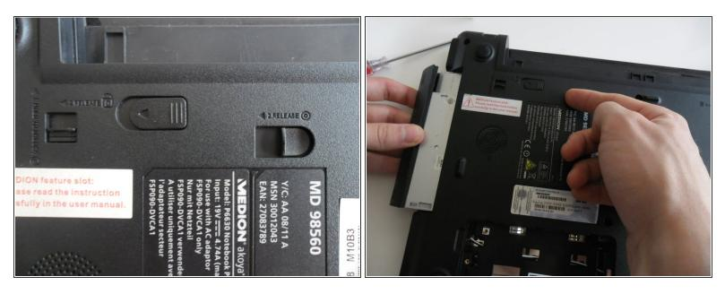
• On the bottom of the case there are 2 sliders, use these to release the optical drive.
