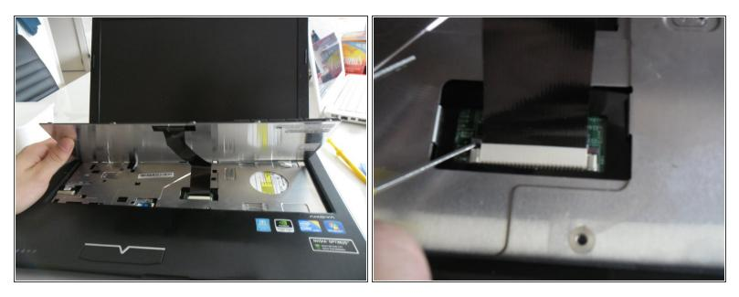
A Be careful when removing the keyboard from the case, it is still attached at the bottom.
