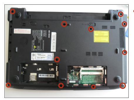
Undo the 11 screws holding the bottom of the case.
