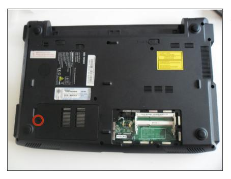
Undo the single screw holding the hard drive lid.
