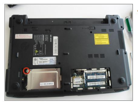
• Undo the single screw holding the hard drive.
