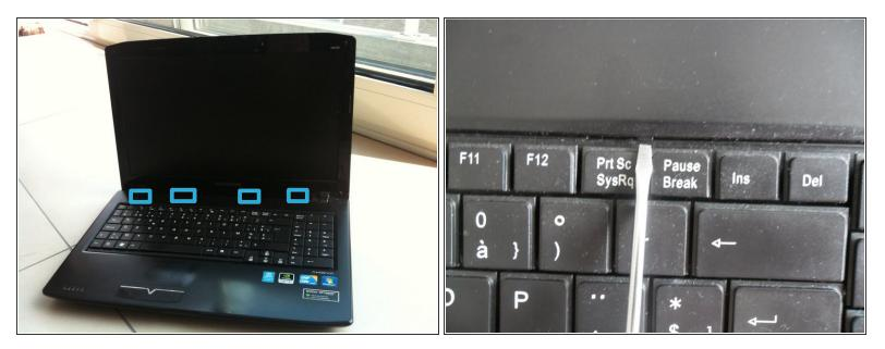
• Push the 4 black tabs located at the top of the keyboard, under the case.
