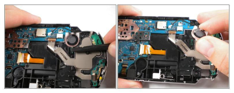
Push the black tab at the bottom of the speaker to pop the speaker out of place, and remove the speaker.
