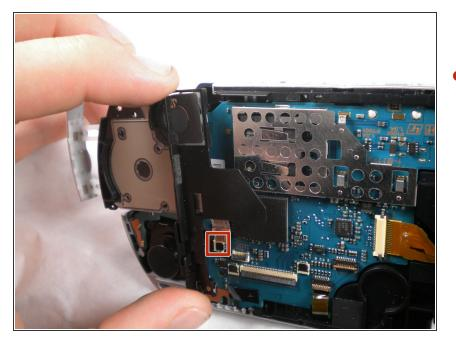
Remove the cable from the connector and remove the entire black piece from the PSP.
