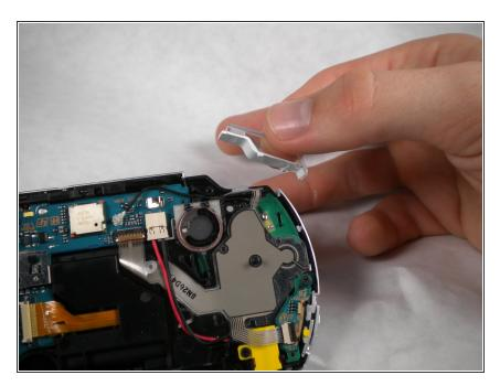
• Remove the 'R' trigger from the PSP.
