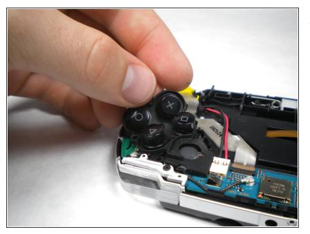
After removing the LCD Screen, the Button Pad should be easy to remove.
