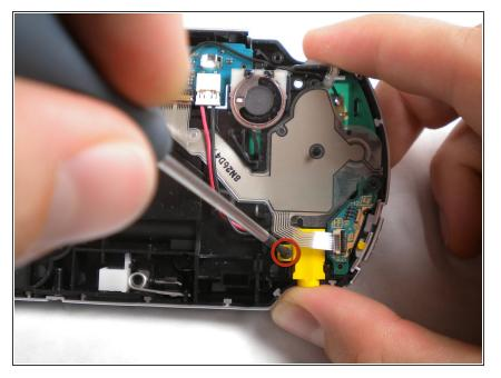
Remove the screw from the power jack.
