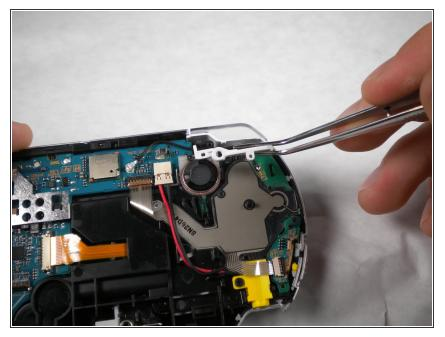
• Remove the white plastic piece that holds the 'R' trigger in place.
