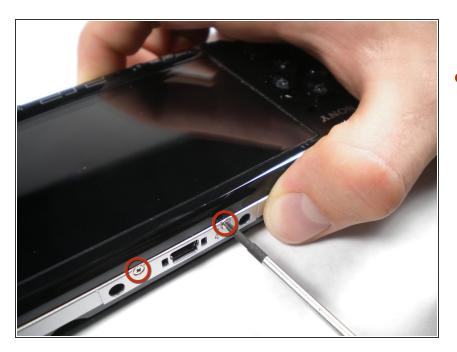
• Next, unscrew the two screws located at the top of the PSP.
