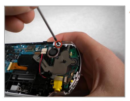
Remove the screw securing the 'R' trigger.
