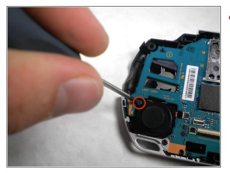
Remove the screw holding the analog stick in place.
