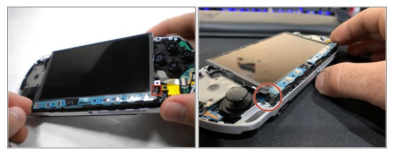
• Push the homebar to the right to release the tab located on the right side of the LCD screen.
