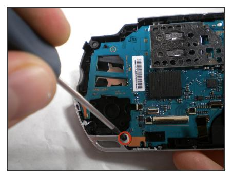
Use a Phillips #00 screwdriver to remove the bottom left screw attached to the PSP
