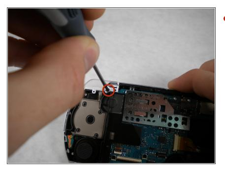
Remove the screw securing 'L' trigger to the PSP.
