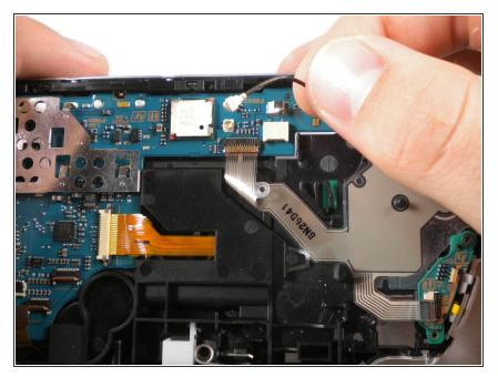
Remove the cable carefully by lifting upwards from port attached to the motherboard.
