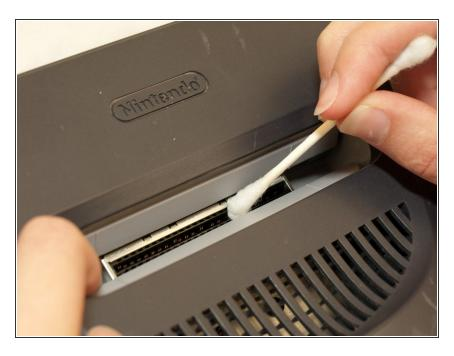
Moist a q-tip with rubbing alcohol.
