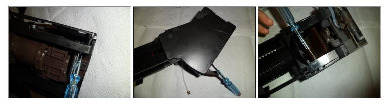
• Now release the side cover. It has 4 clipse. You can open them by pushing with a fingertip or a small screwdriver.
