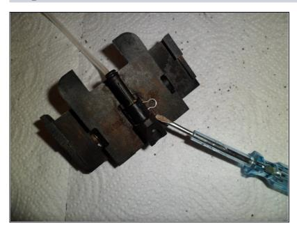
When a lot of water occurs under the brew-group it could be a damaged seal inside the drainage. So I created a Drainage Valve Special, you find it at Coffe Maker Maintenance.
