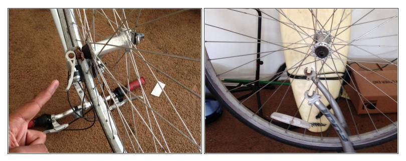
• First, remove the front wheel from the frame by unscrewing the adjustable screw
