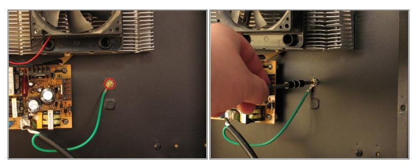
• Remove one 12mm Phillips screw securing ground.
