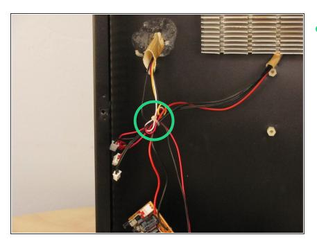
• Cut zip tie binding wires together.
