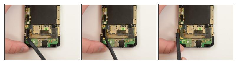
• Pry display assembly connector off of lower logic board.
