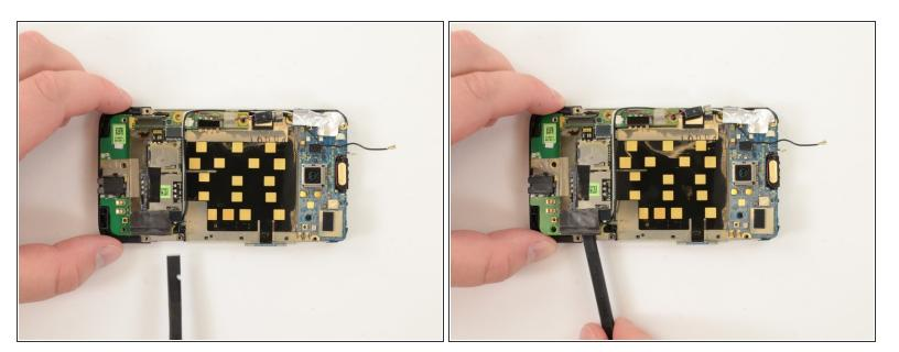
Gently separate lower logic board from mid chassis. The lower logic board is held to the mid chassis by copious amounts of strong adhesive.
