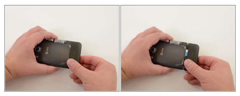
• Remove SIM card cover by simultaneously squeezing cover and pulling it off of the phone.
