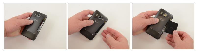
• With the cover removed, the battery will fall freely with a gentle shake.
