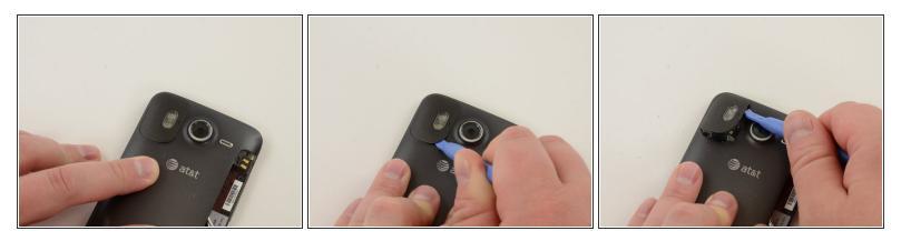
Insert plastic opening tool into gap between GPS cover and back cover of phone. Slide tool along GPS cover and pry the piece off.
