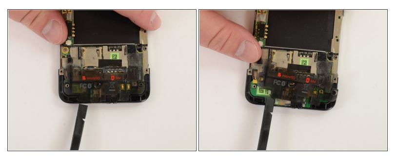
• Apply pressure to the bottom of the plastic logic board shield and it will pop right off.
