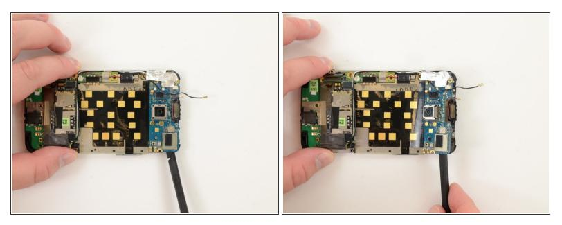
Gently separate upper logic board from mid chassis. The upper logic board is held to the mid chassis by copious amounts of strong adhesive.
