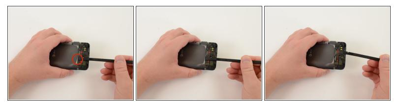
• Remove Micro SD card by pushing it in to the phone. Spring-loaded clasp will release the card.
