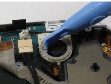
Use the opening tools to press the tab on the left-hand side of the speaker to release it.
