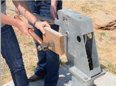
Use a block of wood and hammer to gently tap the axle back into place.
