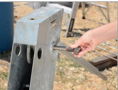
Set the axle punch over the exposed threaded section of the axle.
