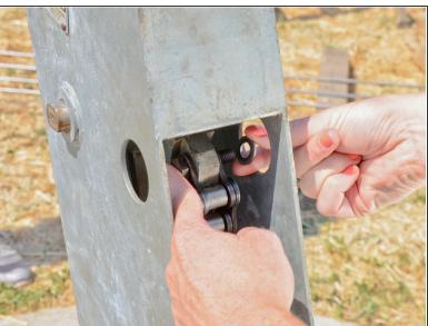
Remove the washer from the chain bolt.
