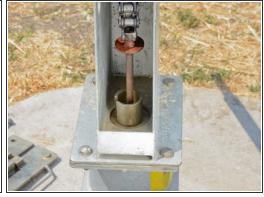
Place the spacer collar around the pump rod below the raised chain, with the beveled side down, and the flat side facing up.
