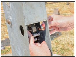
Remove the nut from the chain bolt.
