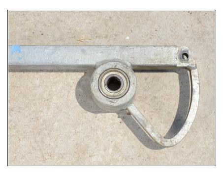
At this point you can inspect the pump handle bearing for damage or excessive wear.
