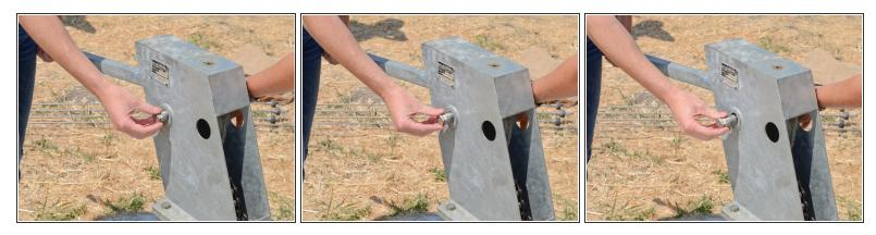
Once the axle is loose, push it through the pump head.
