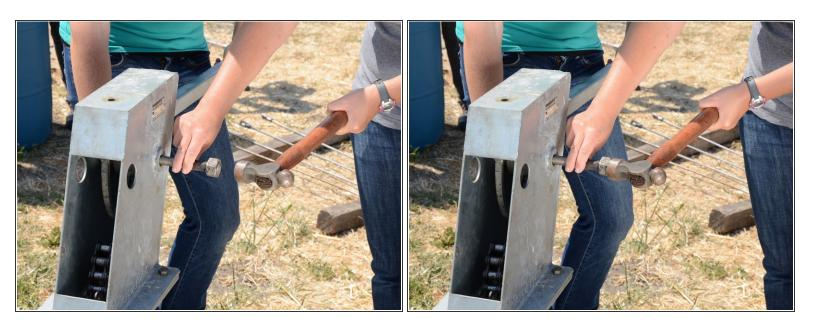
Gently tap the axle punch to push the axle out of the pump head.
