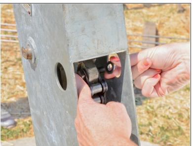
Remove the washer from the chain bolt.
