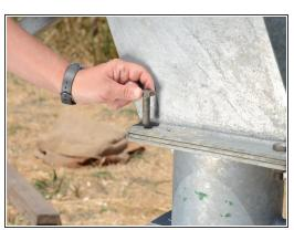
Remove the two bolts and nuts from the handle side.
