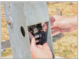
Remove the nut from the chain bolt.
