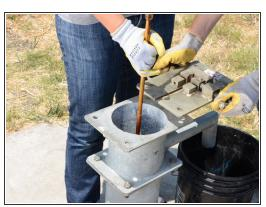
When you reach the final section of the pump rod, remove the rod clamp from the tank.
