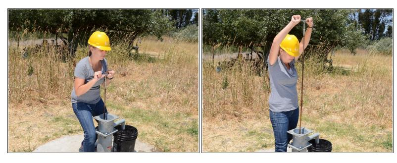
Pull the pump rod up a few feet, past the first joint.
