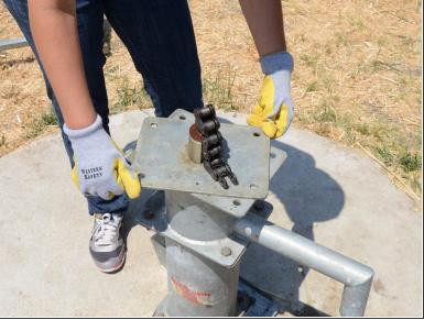
Slightly twist the head flange, until the corners overhang the top of the tank far enough to grab.
