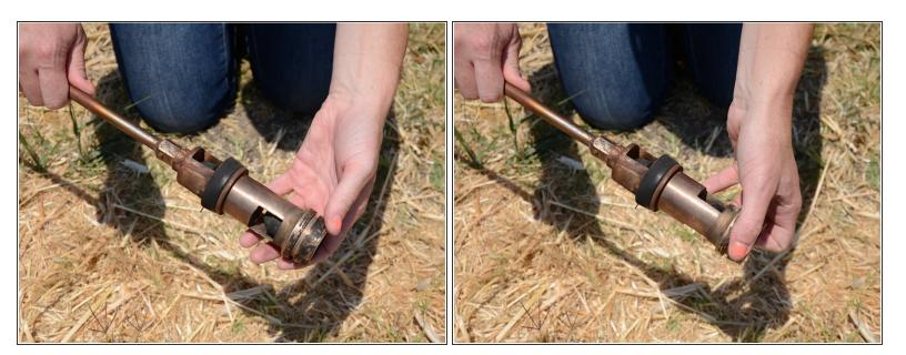
Unscrew the foot valve from the traveling valve.
