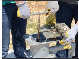
Remove the rod clamp from the tank.
