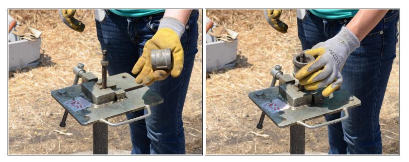
• Place a coupling over the pump rod, on top of the rod vise.
