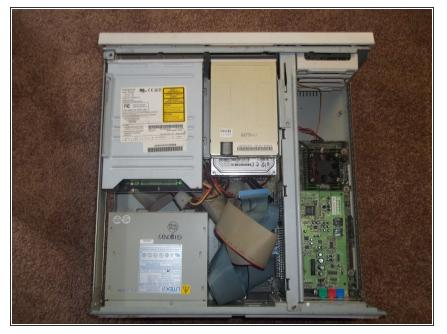
Slide the drive cage back. An easy way to do this is the push on the optical drive from the front.
