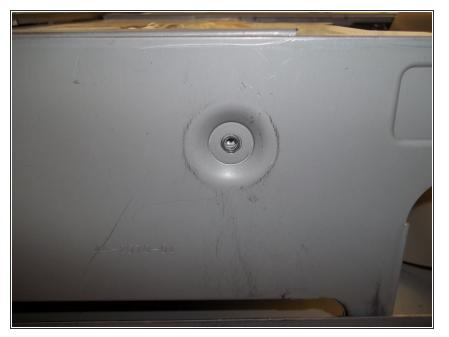
Remove the 1 Philips head screw from the left hand side of the case if there is one. Again, you may need to lubricate this screw.
