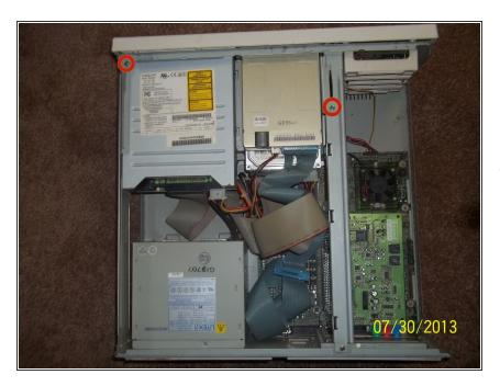
Remove the two Philips head screws with your Philips screwdriver. You may have to
