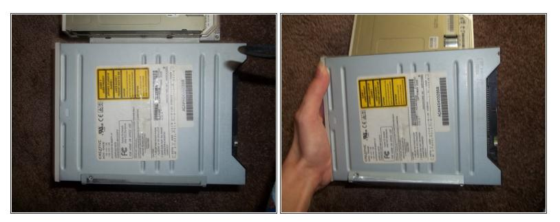
• Slide the optical drive forward and lift it up from the right side, the side closest to the floppy drive.
