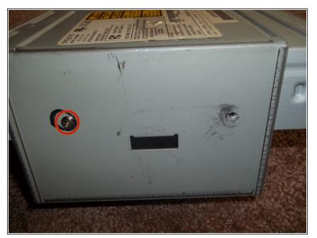
Remove the 1 Philips head screw with your Phillips screwdriver. There should not be a screw in the right hole.
