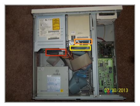
Once the screws are removed, disconnect all cables from the optical drive, hard drive and floppy drive.
