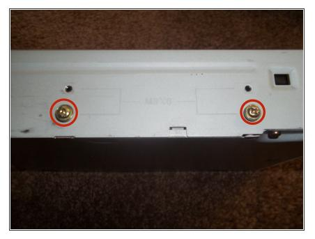
Remove the 2 Philips head screws with your Philips screwdriver. Put these screws onto your new optical drive.
