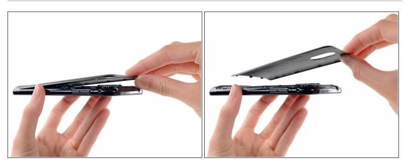
Lift and remove the rear case.
