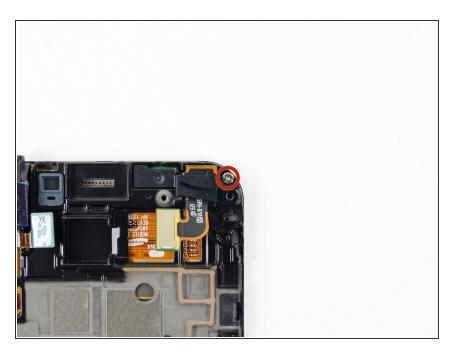
Remove the 2.3 mm Phillips #00 screw securing the front-facing camera bracket to the display assembly.
