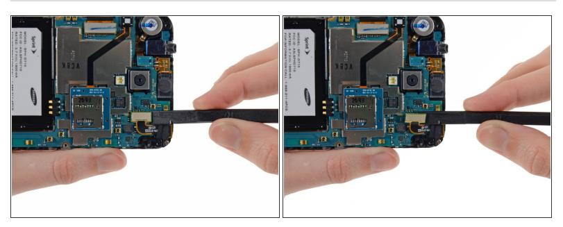
Use the flat end of a spudger to disconnect the front-facing camera cable connector.
