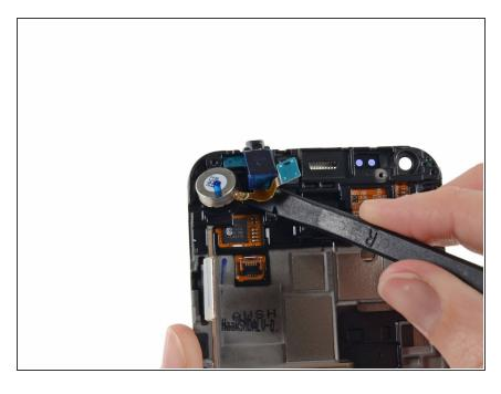
Use the flat end of a spudger to release the headphone jack from the adhesive securing it to the midframe.
