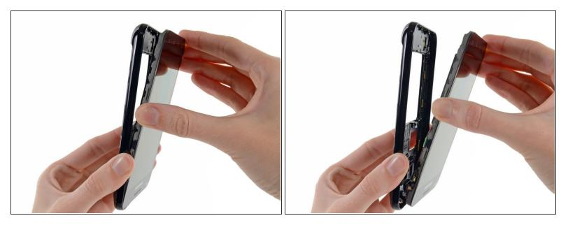
Pull the micro-USB end of the front panel assembly out and away from the midframe and lift up to free it entirely.
