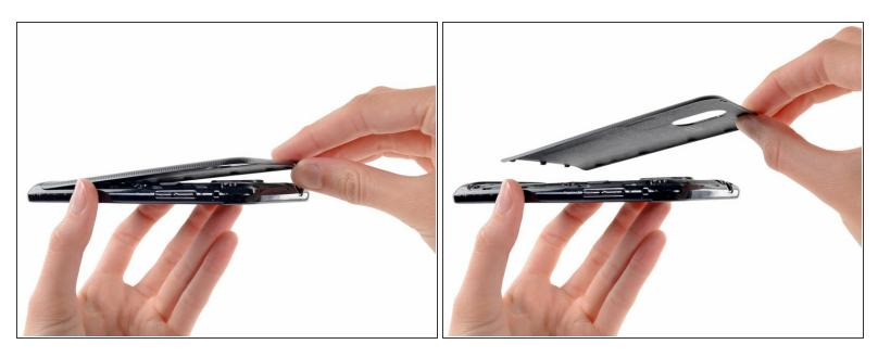
Lift and remove the rear case.
