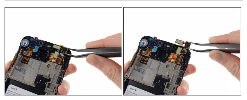
Using a pair of tweezers, or your fingers, remove the front-facing camera/earpiece speaker assembly.
