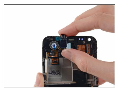
Remove the headphone jack/vibrator assembly from the display assembly.
