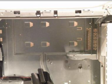
Slide the power supply towards the front of the case, and pull it out. It is a little heavy, so don't drop
