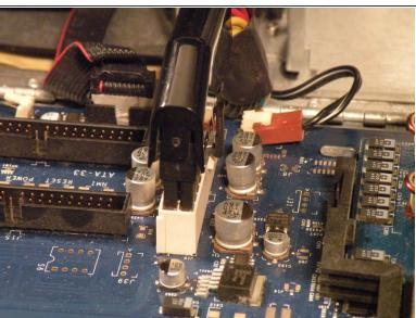
• To remove the power supply connector from the motherboard, push the top end of this clip towards the power supply connector, and pull the connector up and off the motherboard. If the connector seems to be stuck, rock it back and forth a tiny bit to loosen up the connection, then pull up again.
