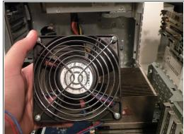
Grab the system fan by its sides and pull it up and out. The system fan is very large and loud, compared to standard sized fans.
