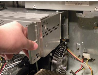
Start removing the optical drive cage by removing its back cover.
