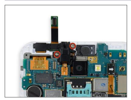
Remove the two 3 mm Phillips #00 screws securing the upper display assembly bracket.
