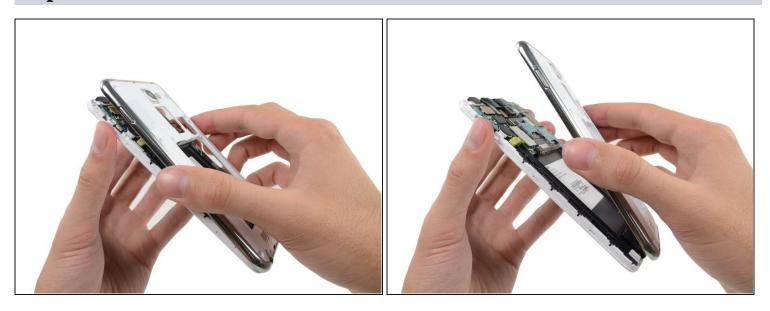
Remove the midframe from the display assembly.
