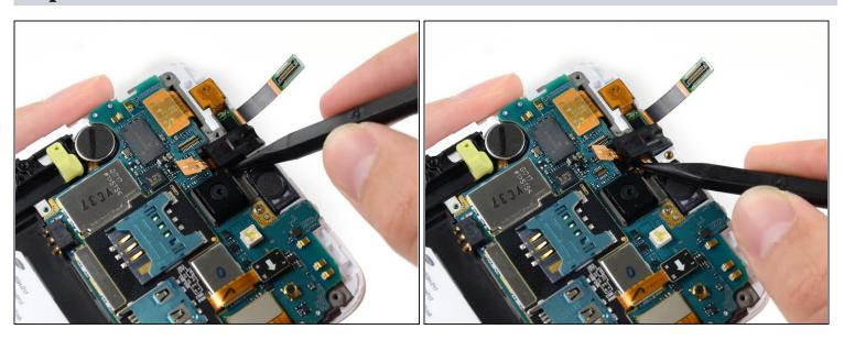
• Use the point of a spudger to pry the headphone jack out of its recess in the display assembly.
