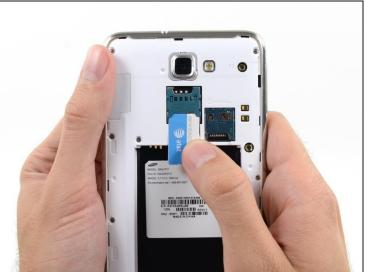
Slide the SIM card out the rest of the way with your thumb and remove it from the device.
