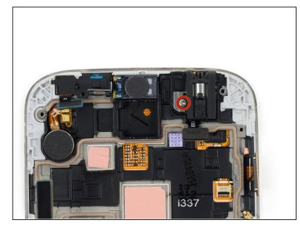
Remove the single 2.4 mm Phillips #00 screw securing the headphone jack assembly to the display assembly.
