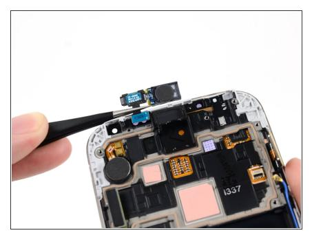
Remove the earpiece speaker assembly from the display assembly.
