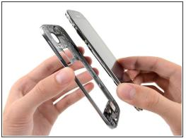
Remove the midframe from the display assembly.
