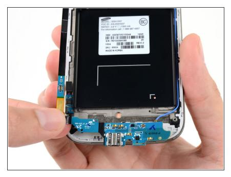
Remove the USB board from the display assembly.
