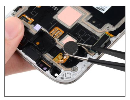
Remove the vibrator from the rear of the display assembly.
