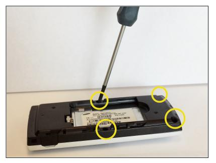
Use a Phillips #00 screwdriver to unscrew the four 3/16" screws holding the black plastic cover of the phone in place.
