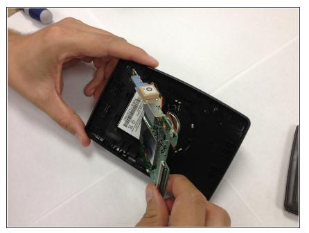
Remove and disconnect the motherboard and battery from the back panel.
