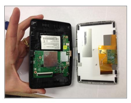
• Release the ribbon cable that connects the two sides.
