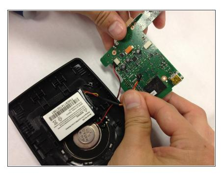
• Attach the motherboard and battery to the new back panel.
